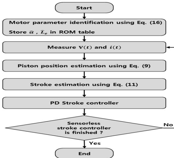
Fig. 7. Flow chart for the stroke control using PIM
