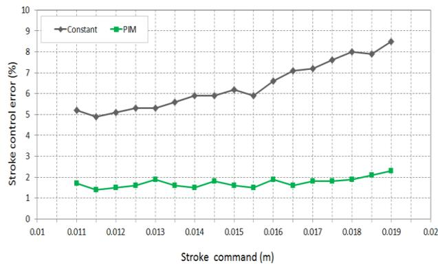
Fig. 11. Stroke control error versus stroke command.
